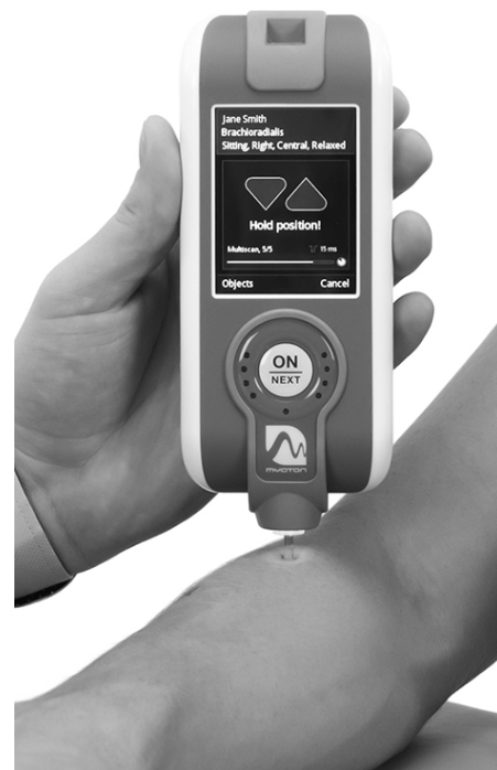
Figure 2: Picture of the handheld device called MyotonPRO in the process of measuring brachioradialis. Published with permission.
